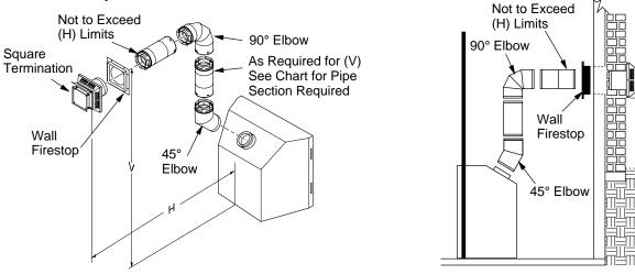
Figure 15 - Horizontal Termination Configuration for Corner Installation Using One 90° Elbow
